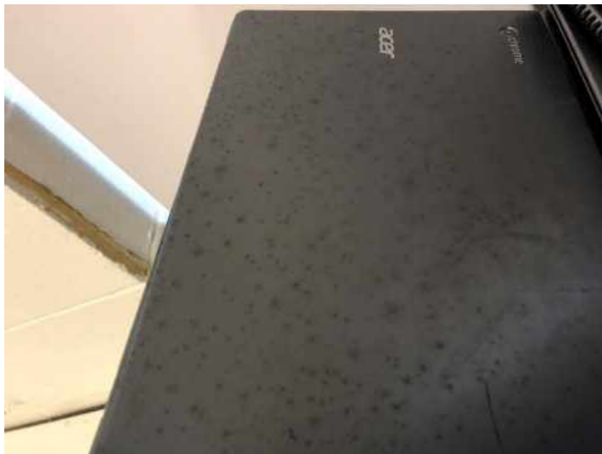
Typical View of Surficial Microbial Growth on Computers (Technology Room – Room 61A)
