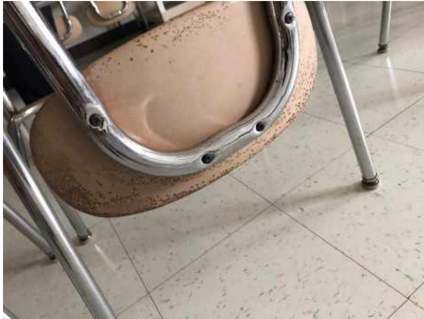
Typical View of Surficial Microbial Growth on Student Chair (Classroom 9)
